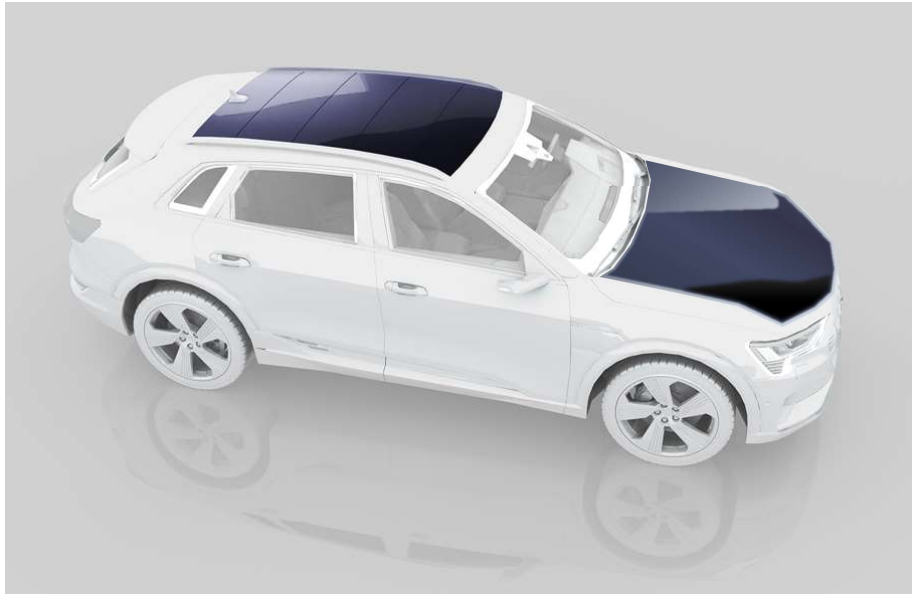
Figure 2: Image of a \text{Cu}_2\text{O} -Si tandem solar cell array installed on an EV.
