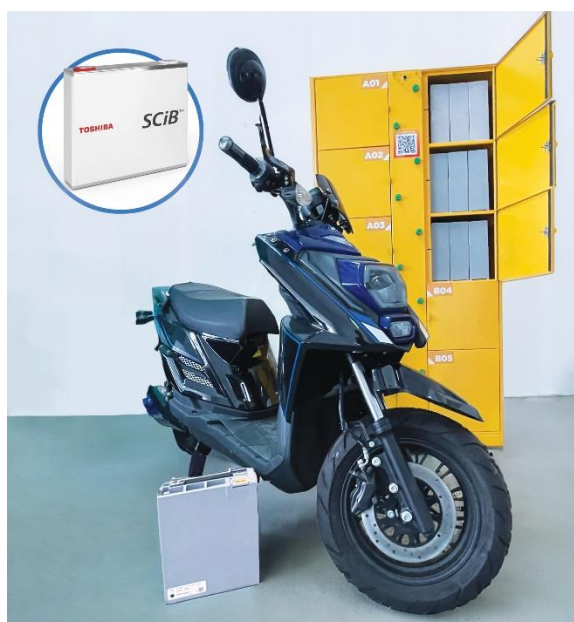
The battery pack using SCiB™ cells and battery charging locker used in the demonstration test, with a motorcycle
